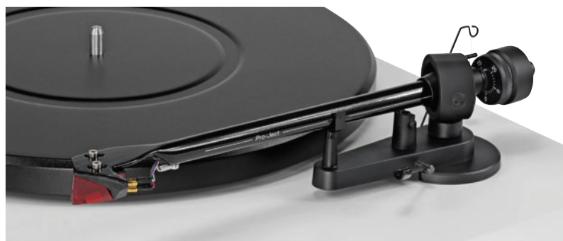
The arm is a one-piece wrapped carbon fibre tube with integral headshell – for lightness and strength. This construction reduces the vibrational modes of a traditional aluminium tube.
